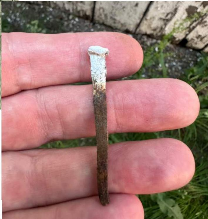
Original cut nail from plank wall construction
