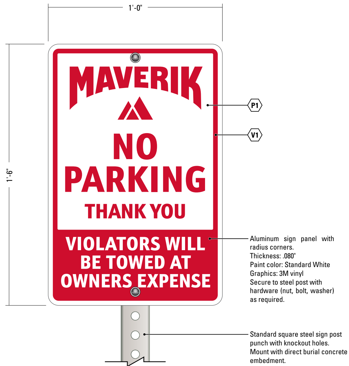
1 SIGN 09 - PANEL DETAIL (TYP.) SCALE: 3" = 1'-0"
